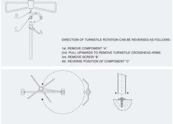
TURNSTILE WILL BE RELEASED FROM THE FLOOR ATTACHMENT BY PULLING IT UPWARDS. SWING THE TURSNTILE TO ALLOW FREE ENTRANCE OF PRODUCTS.
